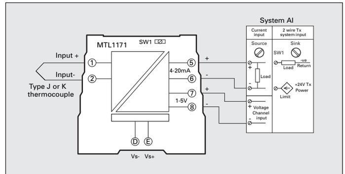
The **MTL1171** is a single channel thermocouple input converter with 4-20mA and 1-5V outputs. Input ranges are switch selectable.
